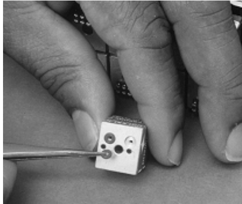
Figure 5.6 DH200 Transducer O-Ring Replacement
